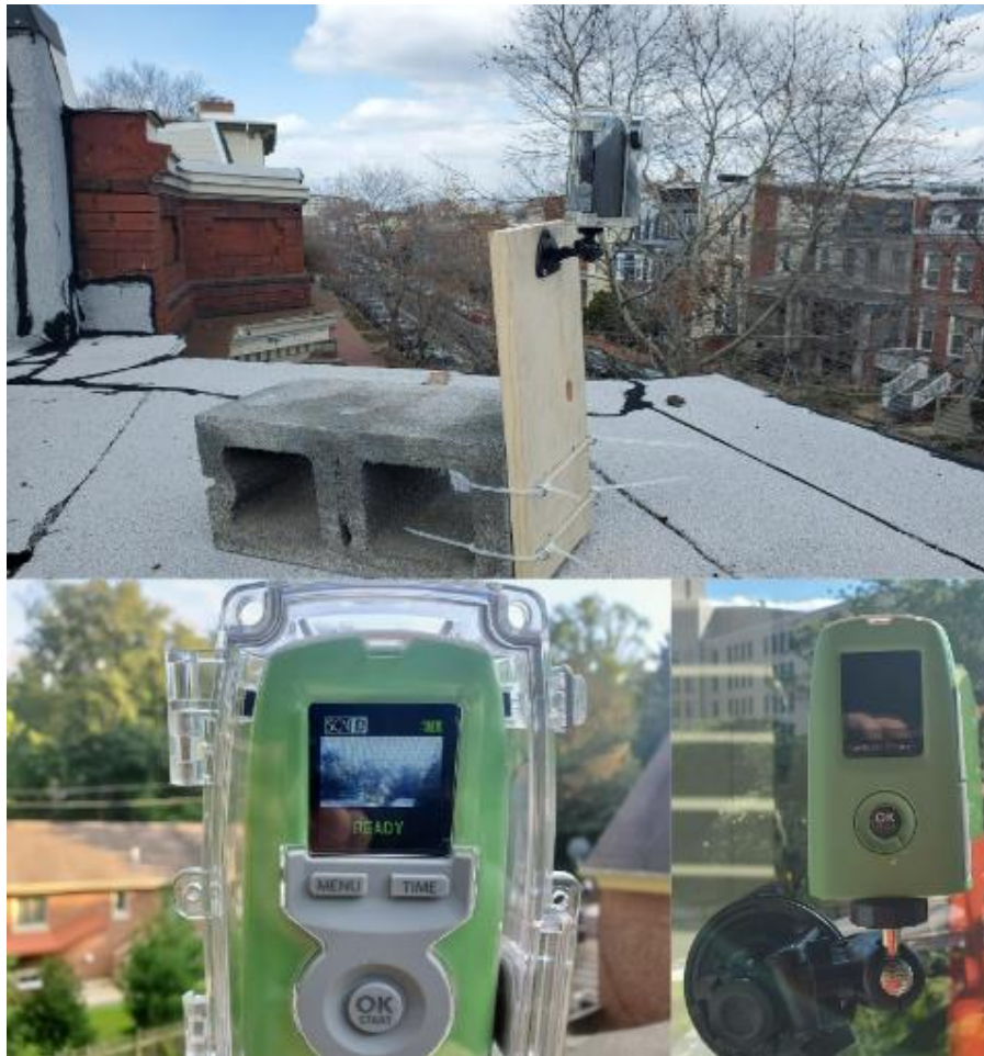
Figure 5. Examples of phenocam set-ups. Top: Outdoor phenocam mount on roof. Bottom Left: Protective case and screen view. Bottom Right: Indoor phenocam suction mount on window.
